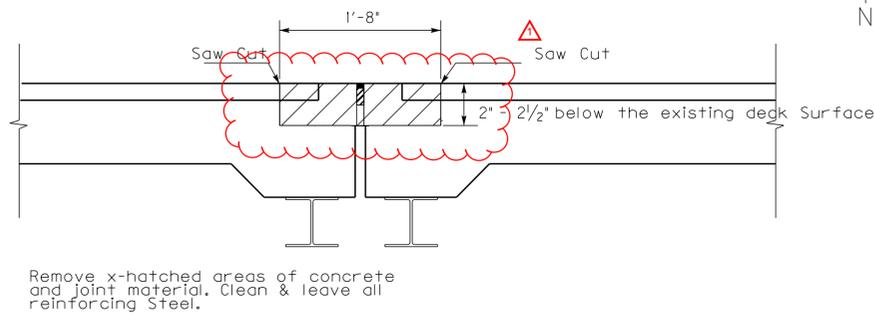
Remove x-hatched areas of concrete and joint material. Clean & leave all reinforcing steel.
